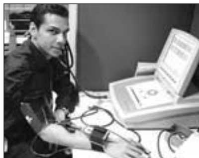
Antonio Leonida uses the Finometer to measure beat-to-beat blood pressure wave shape at the fingertip.
